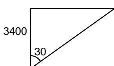
$$\begin{aligned} \tan 30 &= \frac{10v}{3400} \\ v &= \frac{340}{\sqrt{3}} = 196.3 \text{ m s}^{-1} \end{aligned}$$
