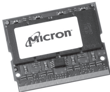
Figure 4-11 144-pin micro-DIMM (photo courtesy of Micron Technology, Inc.)
