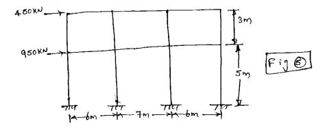
7) Analyse the frame loaded as shown in Fig. 6. by Kani's method and sketch the bending moment diagram.
