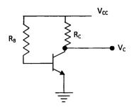
Given;  $V_{CC}$  = volts,  $R_B$  = 400 k $_{\Omega}$ ,  $R_C$  = 1 k $_{\Omega}$ ,  $\beta$  =100,  $V_{BE}$  =0.3 volts.
