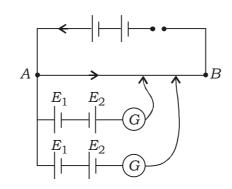
If the balancing lengths for the two combinations of the cells are 250 cm and 450 cm respectively, calculate the ratio of  $E_1$  and  $E_2$ .
